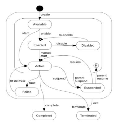
Figure 8.3 - Lifecycle of a Stage or Task instance
