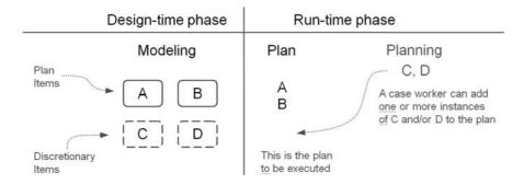
Figure 4.1 - Design-time phase modeling and run-time phase planning
