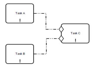
Figure 6.38 - Using Sentry-based connectors to visualize "OR"
